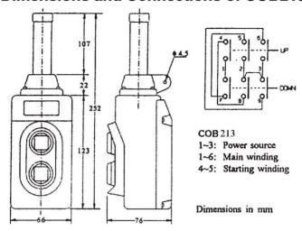
Designed for direct control of single phase electric motors. Since motor current is controlled directly by the pendant switch no extra reversing contactors or costly controls are required.
